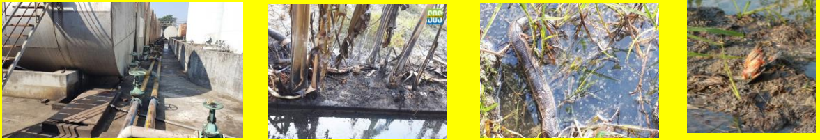
Diesel spill caused by a broken bottom discharge valve of the tank at a military petroleum depot, Quang Hung ward, Thanh Hoa province
