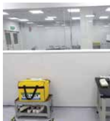
Spill kits equipped at chemical spill risk points of medical equipment factory
