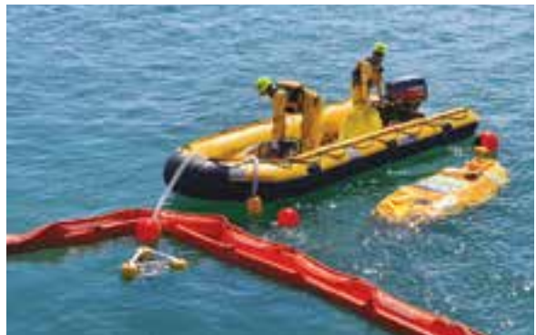
Deploy floating tanks to temporarily store oil-contaminated water recovered from offshore oil spill response activities
