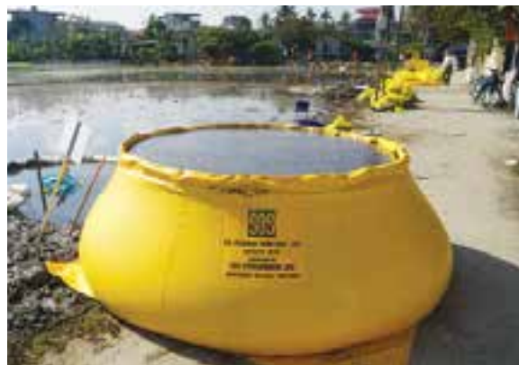
Use open-top temporary storage tank to temporarily store oil-contaminated water recovered from oil spill response activities
