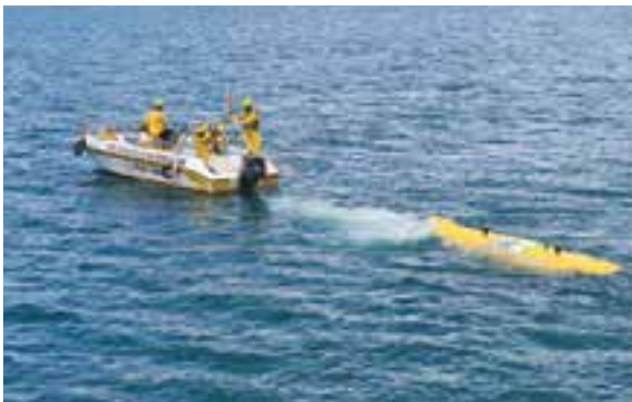
Deploy floating tanks to temporarily store oil-contaminated water recovered from offshore oil spill response activities
