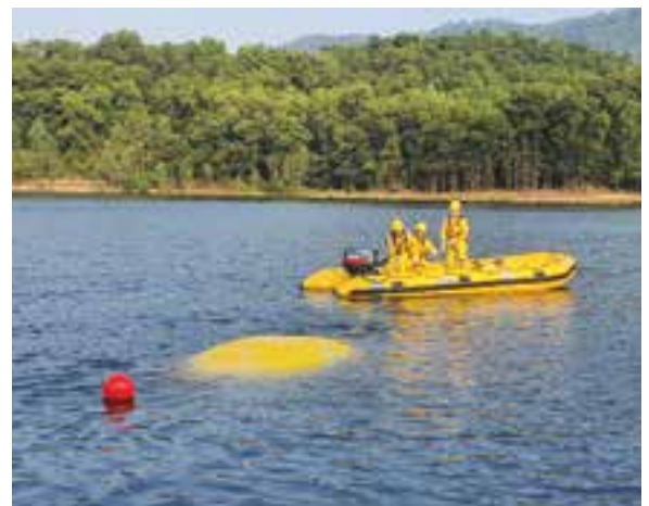
Deploy floating tanks to temporarily store oil-contaminated water recovered from oil spill response activities on rivers and lakes
