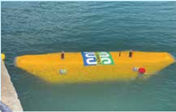
Deploy floating tanks to temporarily store oil-contaminated water recovered from oil spill response activities on rivers and lakes
