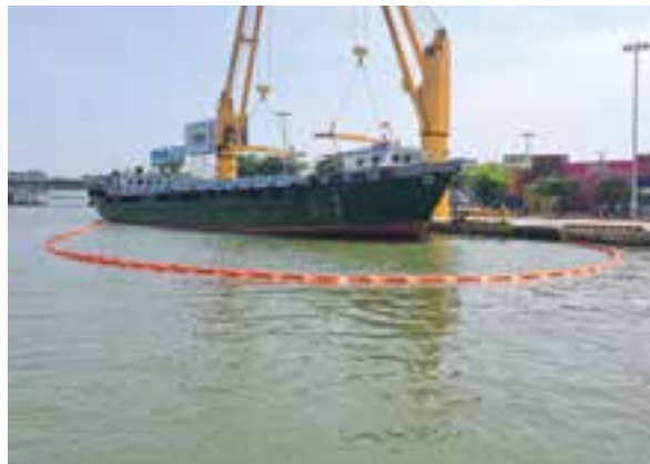
Use oil containment booms to isolate oil spill at port
