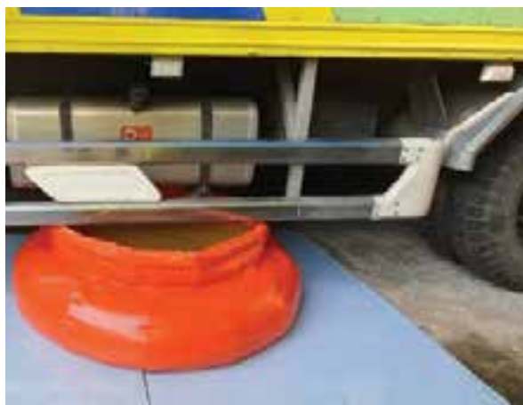
Deploy mobile tank to catch oil leaks under a truck
