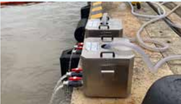
Use mobile oil filtering module to treat oil-contaminated water collected from incident response activities on-site
