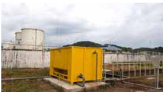
Using oil-contaminated wastewater treatment module to treat oil-contaminated water on-site at petroleum depots
