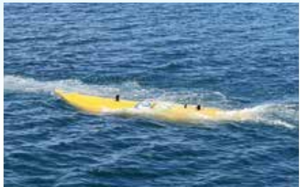
Deploy floating tanks to temporarily store oil-contaminated water recovered from oil spill response activities on rivers and lakes
