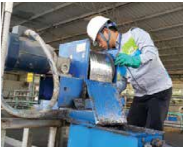
Oil skimmers installed in the oily wastewater collection tanks of mechanical manufacturing factories
