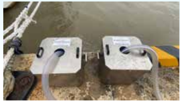
Use mobile oil filtering module to treat oil-contaminated water collected from incident response activities on-site
